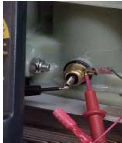
Figure: Thermistor #4 or TH-4 shown with ohm meter probes attached to measure resistance.
