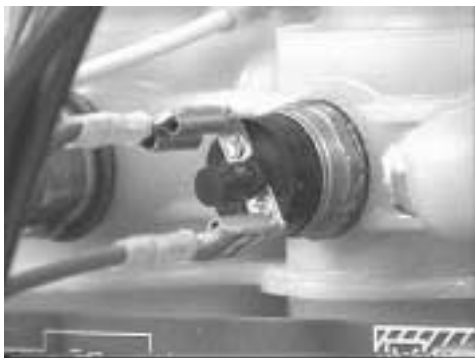
Figure: High limit switch, reset button shown in the middle between the two spade connectors.
